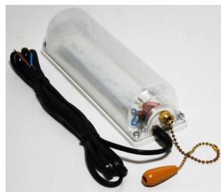
The type SEPS-SLF2 solar light fitting used in this system is a small PVC bulkhead with a 4x1W LED strip module producing a light intensity of 640 lumens and a LED luminous efficacy of 10.6 Watt (65W Incandescent). The light fitting is fitted with a fixed 3m input cable.
