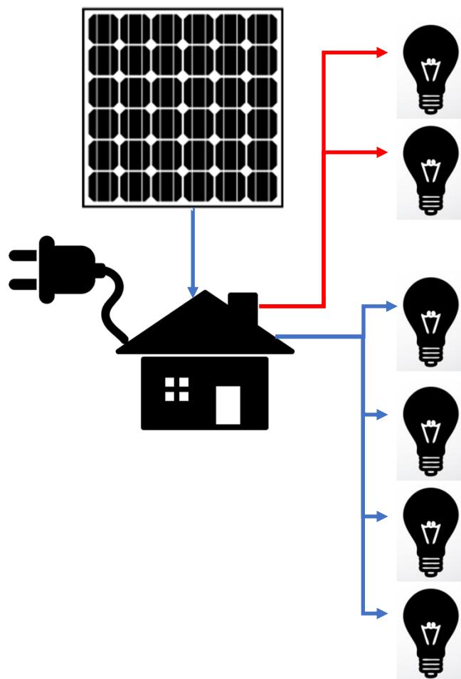
With option one the mains power is installed and enabled. The system will activate the emergency mode and disable two of the outputs on the system. All the outputs can be set for day/night mode or permanent mode. This means that when the system is set to emergency mode the two ports will not function until the mains power is interrupted. If the system does not detect the mains power it will allow the lights connected to the emergency outputs to go live and allow for the light to switch on.
