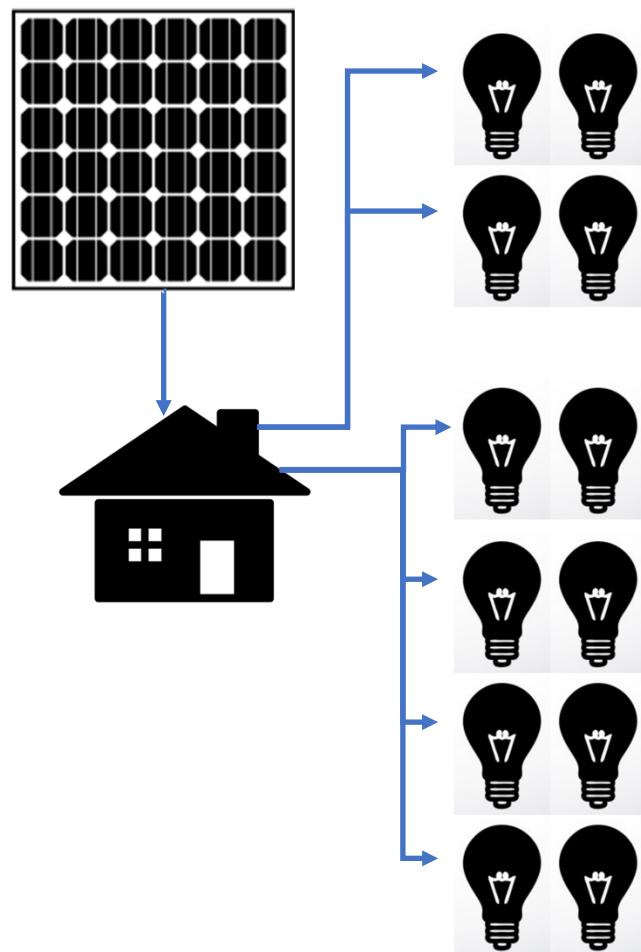
With option two being select all the ports will function based on the mode selected for the outputs. If permanent on mode is selected the lights will remain on and never switch off. If the day/night mode is selected the system will only activate all the ports once the sun sets.
