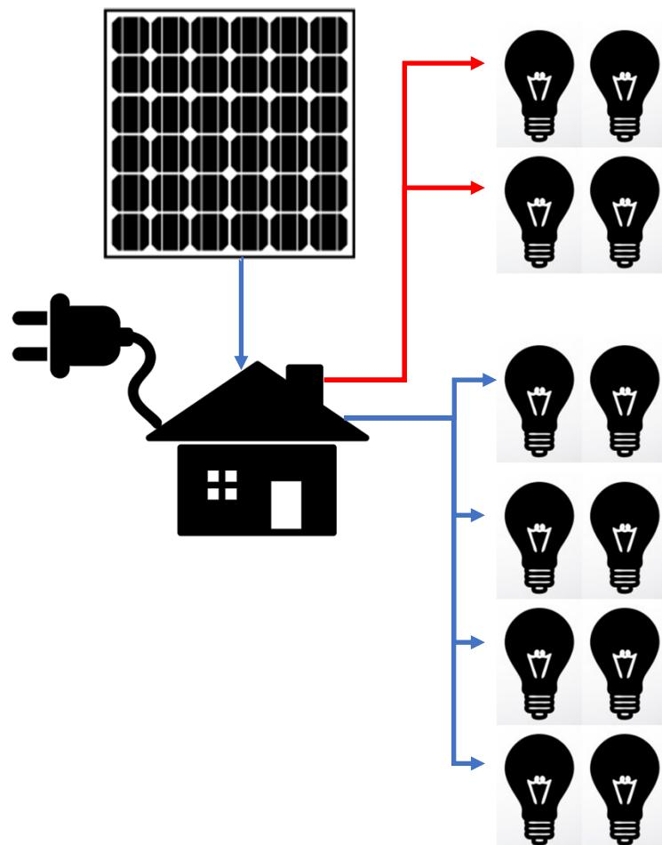
With option one the mains power is installed and enabled. The system will activate the emergency mode and disable two of the outputs on the system. All the outputs can be set for day/night mode or permanent mode. This means that when the system is set to emergency mode the two ports will not function until the mains power is interrupted. If the system does not detect the mains power it will allow the lights connected to the emergency outputs to go live and allow for the light to switch on.
